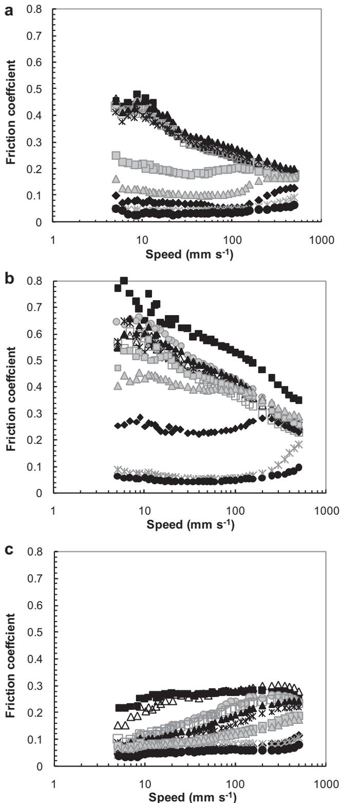
**Fig. 1.** Friction coefficient measured at load  $W = 5$  N with (a) silicone, (b) neoprene or (c) Teflon for milk samples with different fat content. The symbols correspond to: ■ 0.06; △ 0.15; ○ 0.3; □ 0.5; ▲ 0.7; ✱ 1; ▣ 2; ▲ 3; ◆ 4; ✱ 6.5; ● 8.7%.
