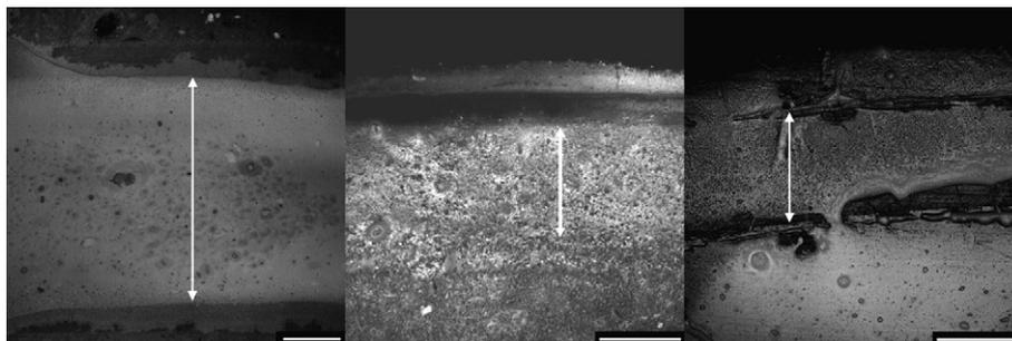
**Fig. 3.** Confocal laser scanning microscopy images of three different rubbers (left image, silicone; middle image, neoprene; right image, Teflon) after processing 3.5% milk in a Mini Traction Machine. Scale bar corresponds to 250  $\mu\text{m}$  for silicone and 750  $\mu\text{m}$  for neoprene and Teflon.
