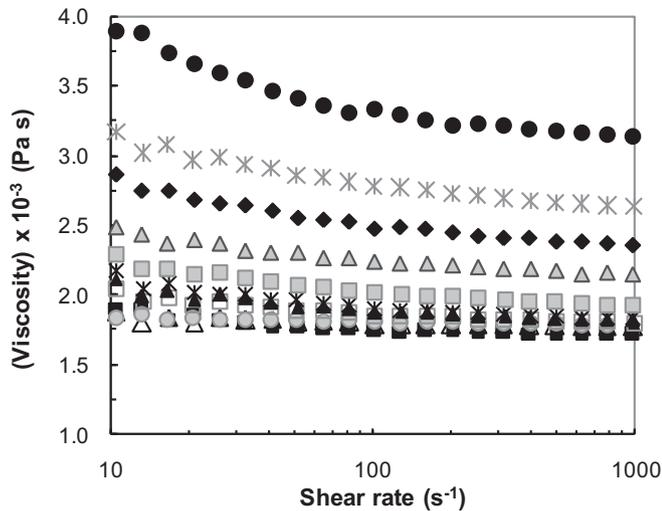
**Fig. 2.** Viscosity as a function of the shear rate for milk samples containing different fat content. The symbols correspond to: ■ 0.06; △ 0.15; ○ 0.3; □ 0.5; ▲ 0.7; ✱ 1; ▽ 2; ▲ 3; ◆ 4; ✱ 6.5; ● 8.7%.
