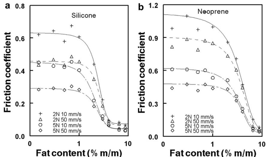
**Fig. 5.** Friction coefficient as a function of fat content for (a) silicone and (b) neoprene. Symbols correspond to different experimental conditions: +, load ( $W$ ) of 2 N and speed ( $U$ ) of  $10 \text{ mm s}^{-1}$ ;  $\Delta$ ,  $W = 2 \text{ N}$ ,  $U = 50 \text{ mm s}^{-1}$ ;  $O$ ,  $W = 5 \text{ N}$ ,  $U = 10 \text{ mm s}^{-1}$ ;  $\diamond$ ,  $W = 5 \text{ N}$ ,  $U = 50 \text{ mm s}^{-1}$ . Lines are fits to a sigmoidal function.
