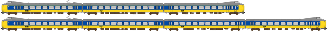
FIGURE 3.3: Two train units of the same train type, ICM, but different subtypes: the top train unit consists of three carriages (ICM-3); the bottom one has four (ICM-4).
