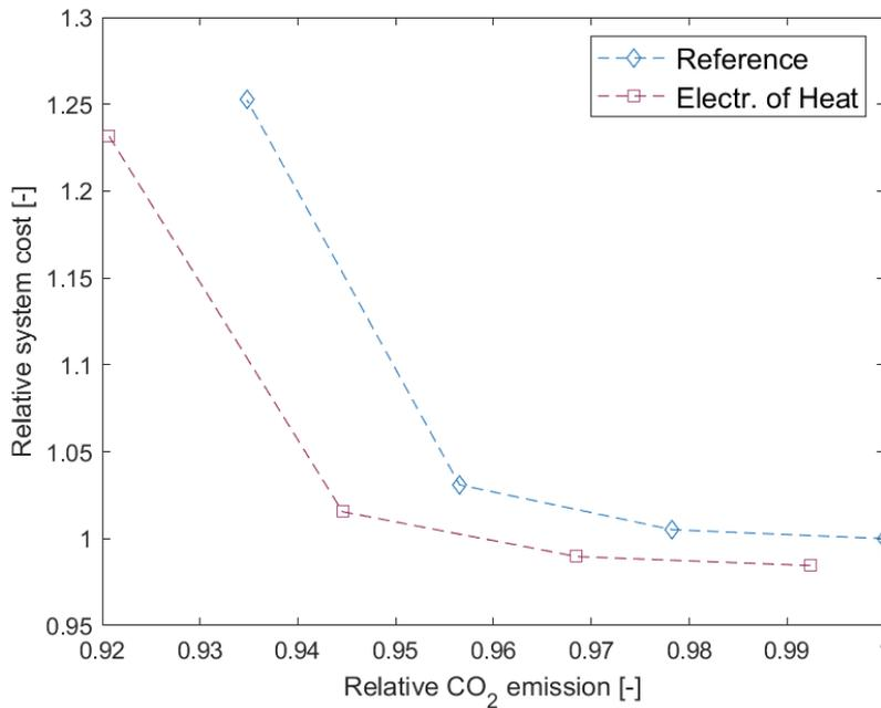
Figure 15: Pareto front of CO<sub>2</sub> emissions and system cost, relative to the minimum cost design of the reference scenario, for the electrified heat scenario
