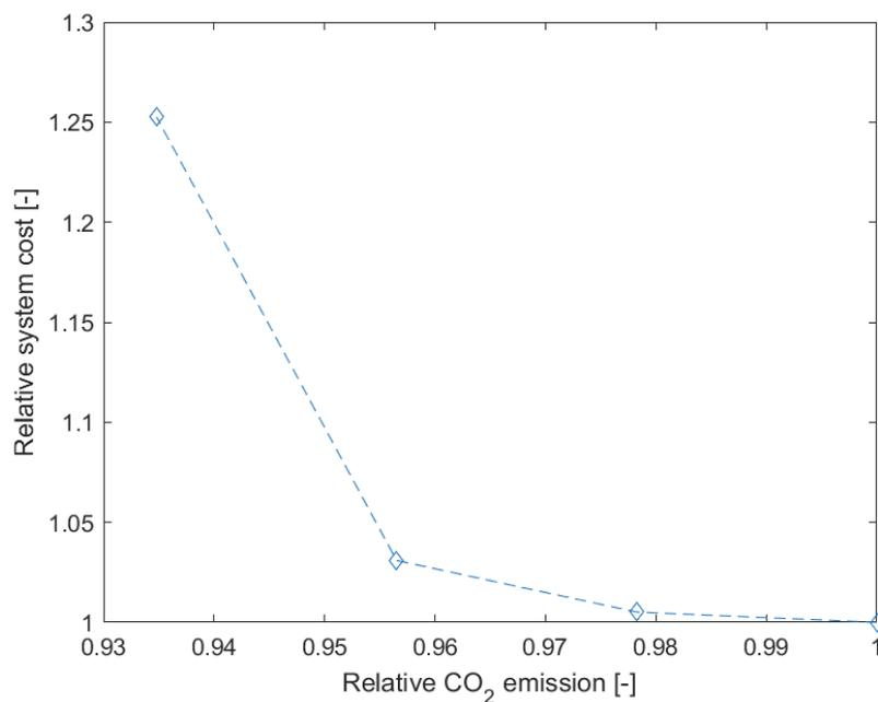
Figure 13: Pareto front of CO<sub>2</sub> emissions and system cost, relative to the minimum cost design, for the reference scenario
