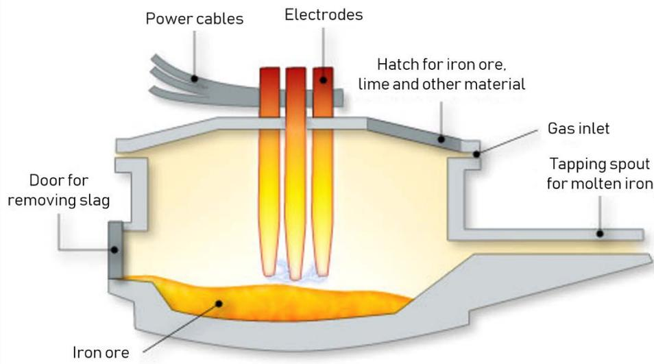
Figure 9: Sketch of an electric arc furnace (EAF) adapted from [12]
