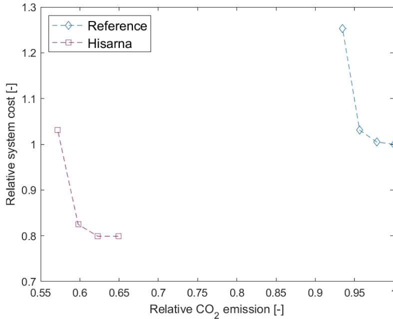
Figure 17: Pareto front of CO<sub>2</sub> emissions and system cost, relative to the minimum cost design of the reference scenario, for the Hisarna scenario
