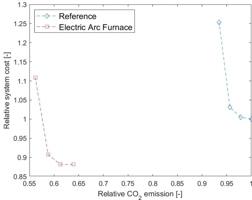
Figure 19: Pareto front of CO<sub>2</sub> emissions and system cost, relative to the minimum cost design of the reference scenario, for the Electric Arc Furnace scenario
