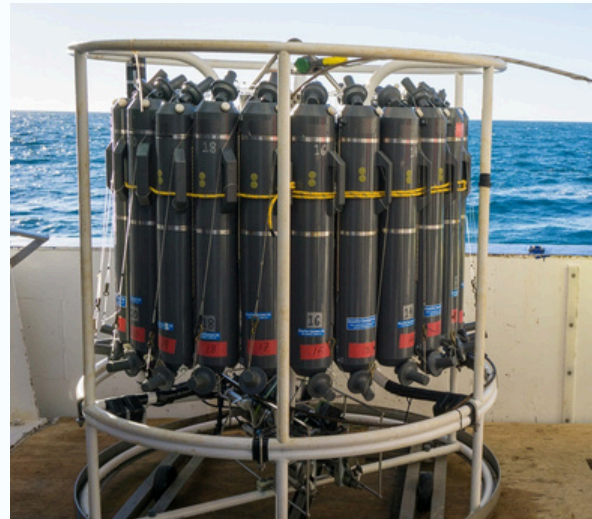
Figure 3. The CTD on the RV Pelagia we deployed to track the temperature and salinity profiles of the NBC ring.
