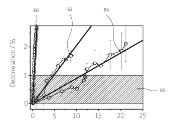
Illustration from the patent application: Decorrelation vs. temperature change. Temperature compensated glass ceramic (84) is much more stable against temperature changes than ordinary glass (80) or non-compensated glass ceramic.
