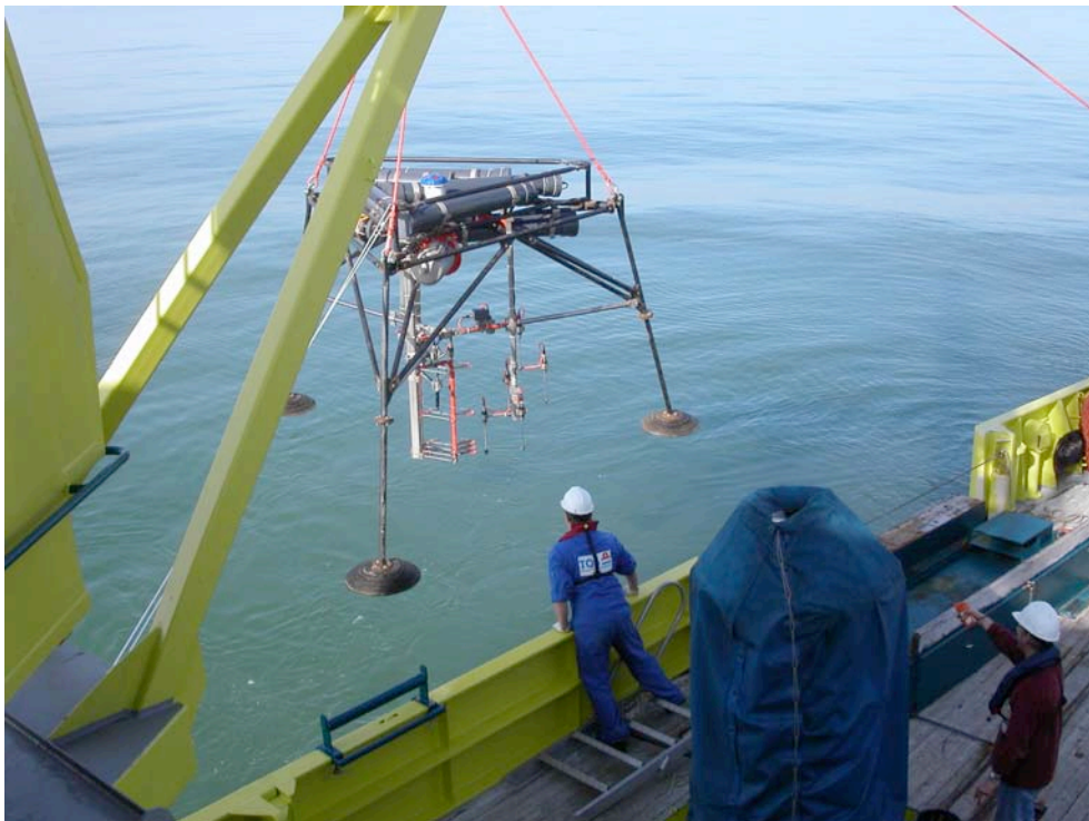
Figure 14. Deployment of HSM tripod (HSM = Hydrodynamics, Sediment transport and micro-Morphology of the seabed) in the Noordwijk transect during the SANDPIT project.
