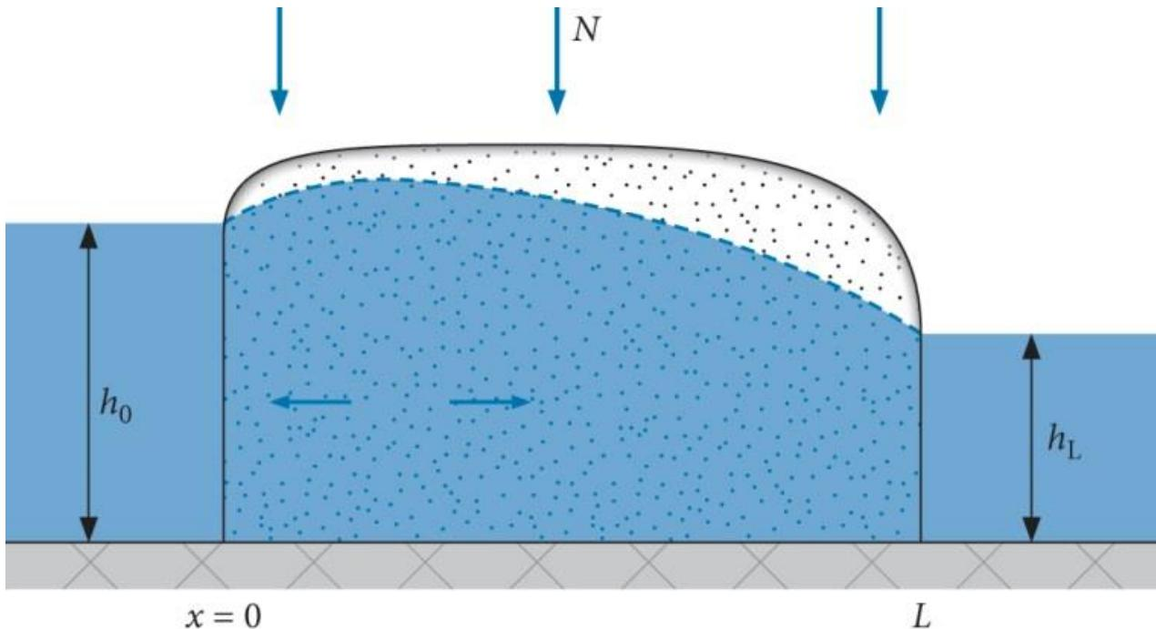
$$Q_x' = -K \left( h \frac{dh}{dx} \right)_x \quad Q_{x+\Delta x}' = -K \left( h \frac{dh}{dx} \right)_{x+\Delta x} \quad Q_{x+\Delta x}' - Q_x' = -K \frac{d\left( h \frac{dh}{dx} \right)}{dx} \Delta x$$
