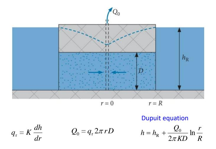
M1-5: hydraulic head *h* decreases with increasing x – minus sign in Darcy's law, linking Q' > 0 with dh/dx < 0 M6-7: hydraulic head *h* decreases with decreasing r – no minus sign in Darcy's law, linking Q' > 0 to pumping
