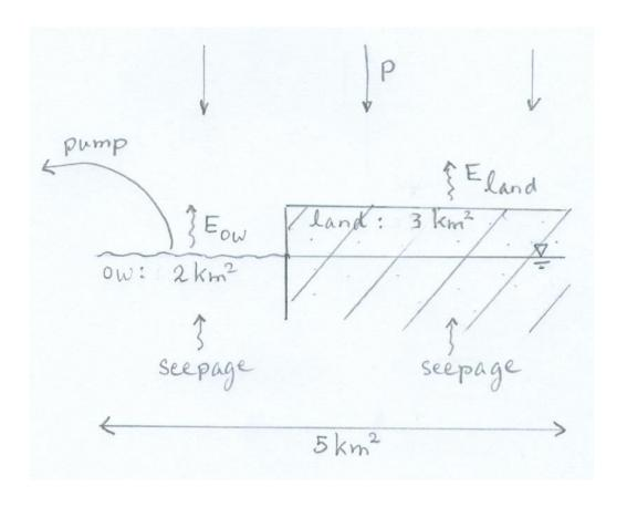
Water balance:  $P + seepage = E_{actual} + pump + (\Delta S/\Delta t)$
