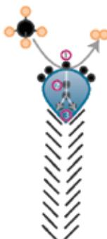
Figure 1: Schematic representation of the decomposition of methane. 1) Decomposition of methane at the surface. 2) Transport of carbon through the metal. 3) Deposition carbon in graphitic layers. Adapted from<sup>[1]</sup>
