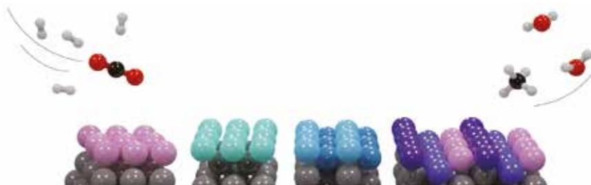
Figure 1: Schematic representation of CO<sub>2</sub> methanation over four nickel facets. Surface atoms with a same structural identification are represented with matching colors.
