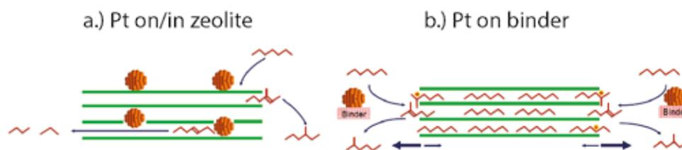
Figure 1: Schematic representation of hydroconversion of n-heptane over a Pt/zeolite/binder bifunctional catalyst with a.) Pt nanoparticles on/in a zeolite crystal, and b.) Pt nanoparticles on a binder material (typically  $\gamma$ - $\text{Al}_2\text{O}_3$ ).
